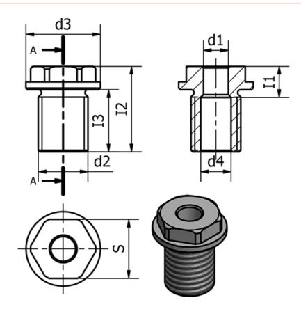
Tightening torque in Nm = 90
